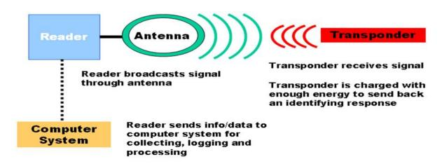
Fig2: How RFID Works
