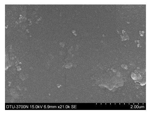
Sample 1- Pure hydrogel formed by Dextran-maleic acid and N-isopropylacrylamide.
