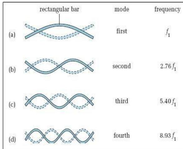
Fig 2. Example of Vibrational Modes
