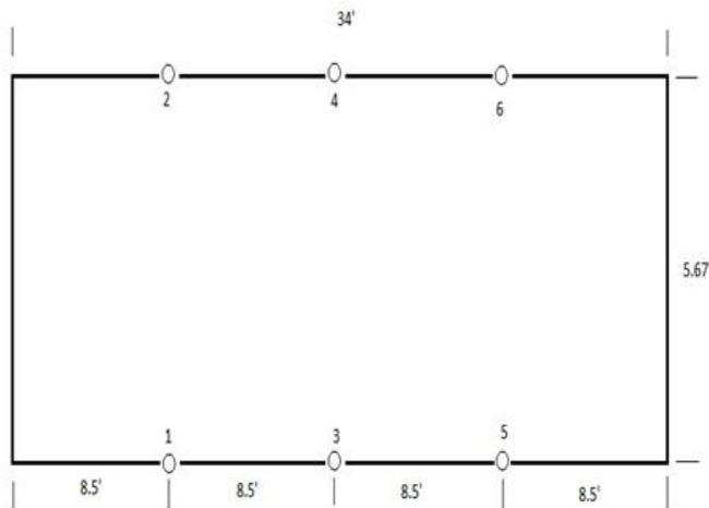
Fig 12. Pedestrian Bridge Sensor Layout
