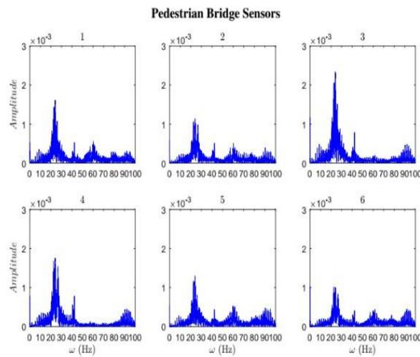
Fig 22. Group of Two Unsynchronized Walking Excitation Response
