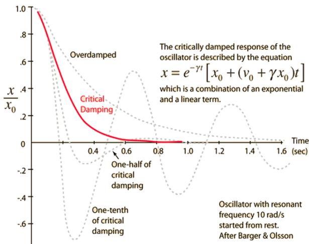
Fig 5. Critical Damping
