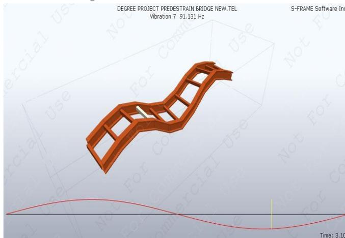
Figure 35: Fourth Mode Shape (Vertical), at 91.13 Hz with energy of 15.34%
