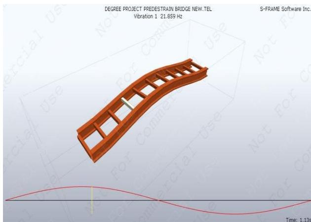
Fig 32. First Mode Shape (Vertical), at 21.86 Hz with energy of 77.34%
