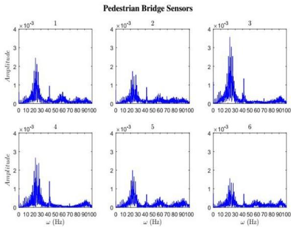
Fig 20. Group of Two Synchronized Walking Excitation Response
