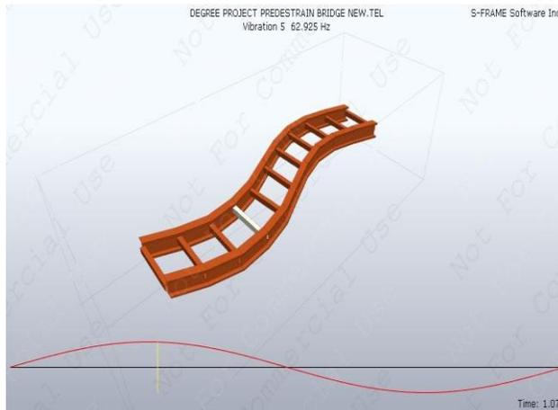
Fig 34: Third Mode Shape (Torsional), at 62.92 Hz with minimum energy
