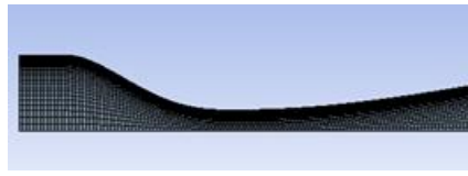
Figure II. Meshed model of an axisymmetric nozzle
