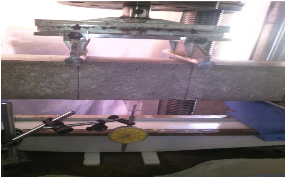
Figure. 7 - Load of Bamboo as Reinforced Beam
