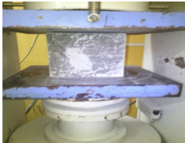
Figure. 4 -Compression Test onCube
