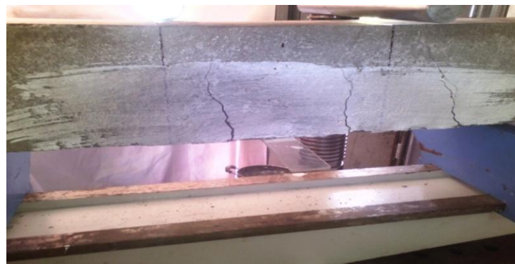
Figure.12 - Crack Pattern of the Beam Specimen
