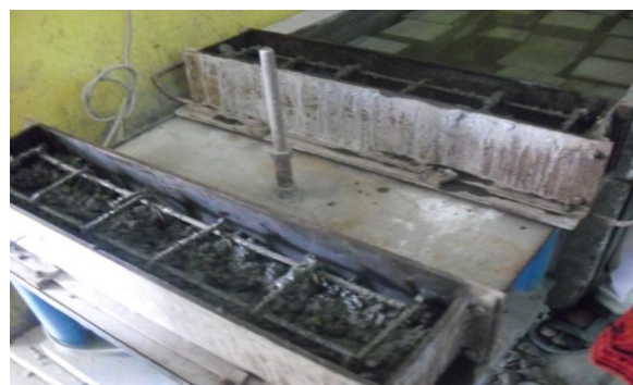
Figure. 3 - Casting of Beam Specimen
