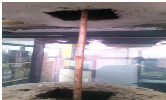
Figure. 5 - Tension Test on Bamboo
