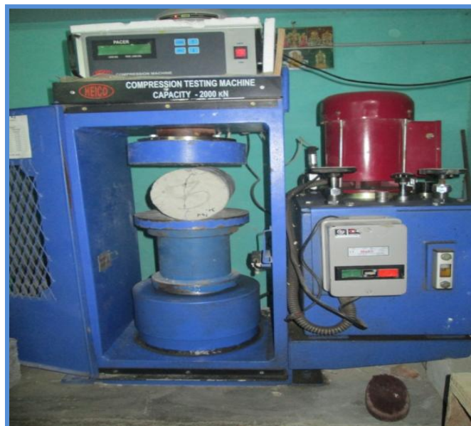
Experimental set up of Split Tensile Strength Test
