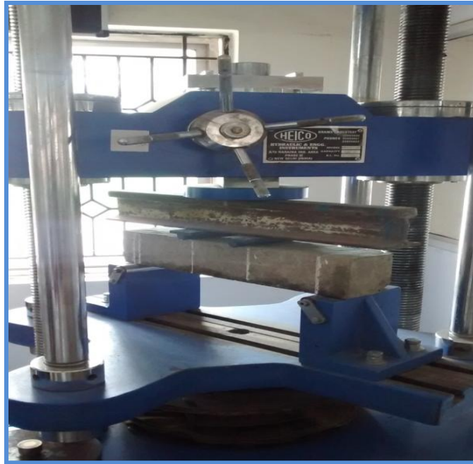
Flexural strength test on prism
