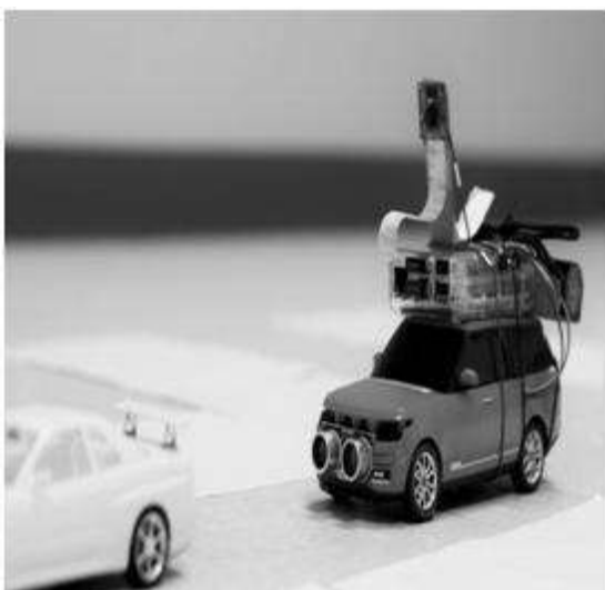
Figure 5. (a) Front collision avoidance system distance measurement (b) front collision avoidance system applying break.
