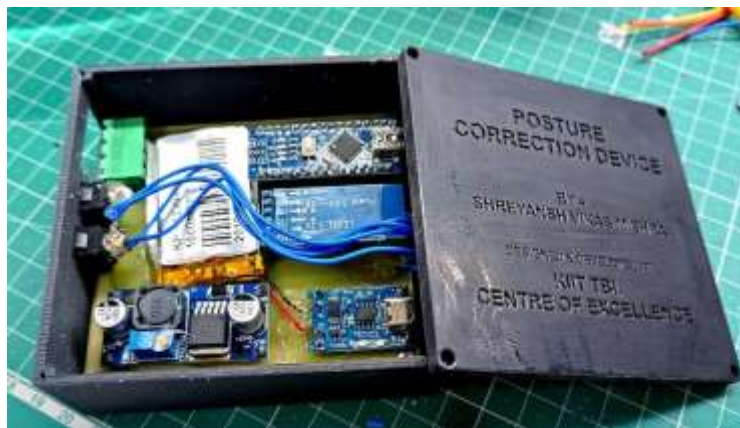
Figure 18: Inside view the Device Casing showing electronics components
