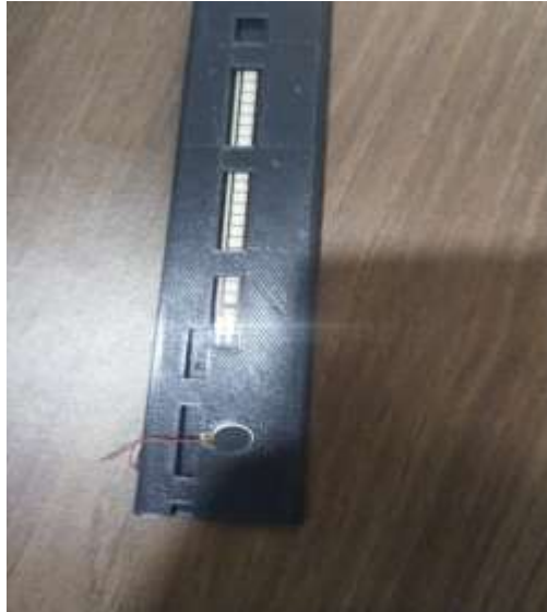
Figure 17: 3D Printed Flexible Casing showing Flex Sensor & Vibrator
