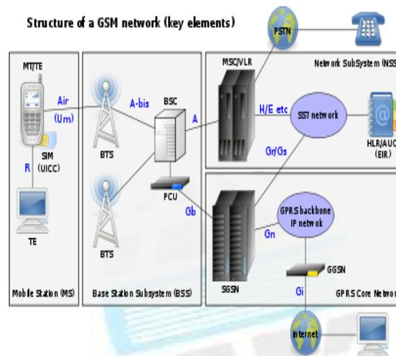
Structure of a GSM network
