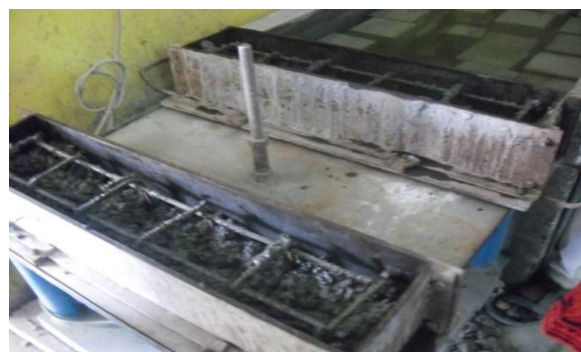
Figure. 3 - Casting of Beam Specimen
