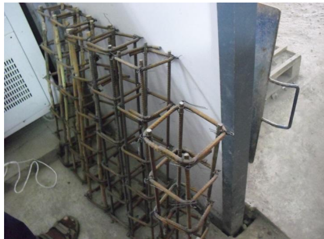
Figure. 1 - Bamboo as Reinforcement in Beam
