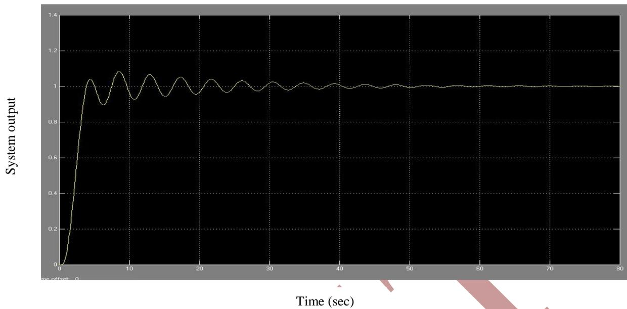
Figure : 8 Step response of process  $P_1(s)$  with conditional integration
