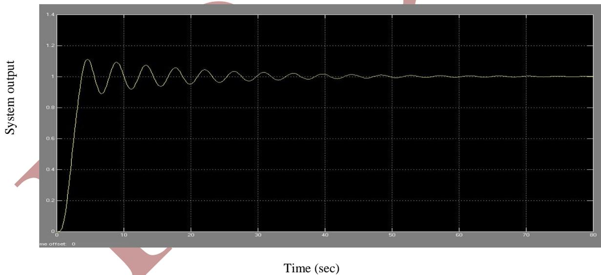
Figure : 7 Step response of process  $P_1(s)$  with back calculation
