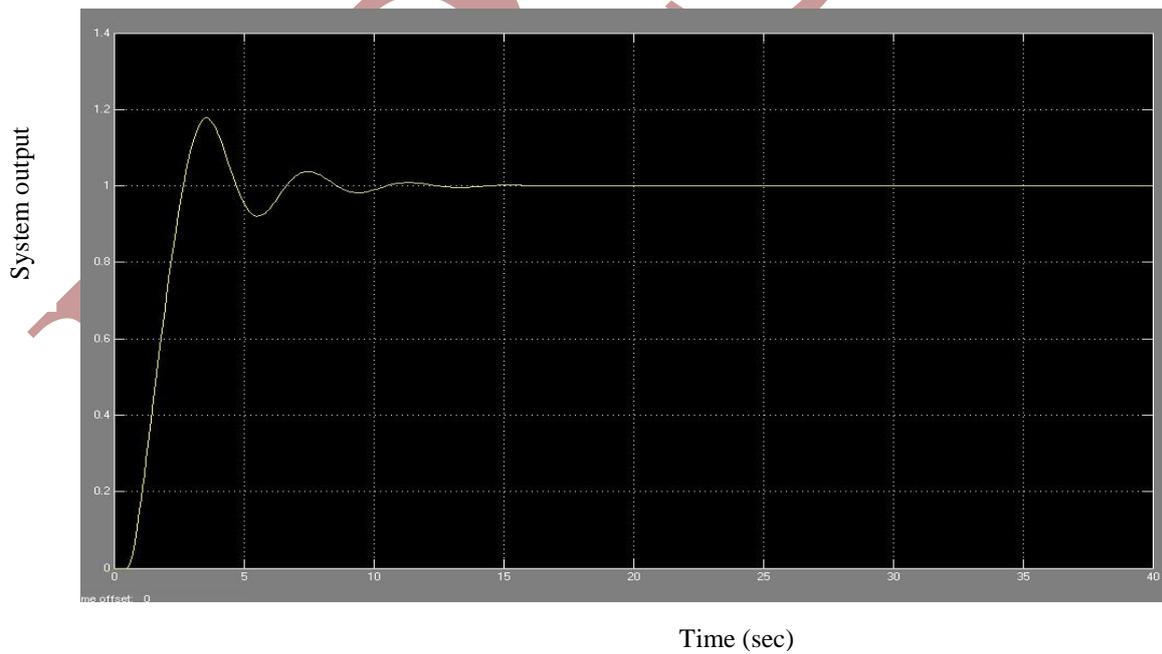
Figure : 3 Step response of process  $P_1(s)$  with back calculation
