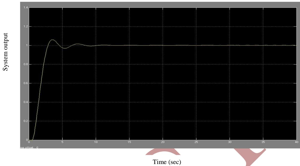
Figure : 4 Step response of process  $P_1(s)$  with conditional integration
