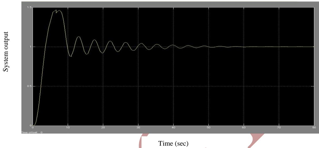
Figure : 6 Step response of process  $P_1(s)$  without anti-windup
