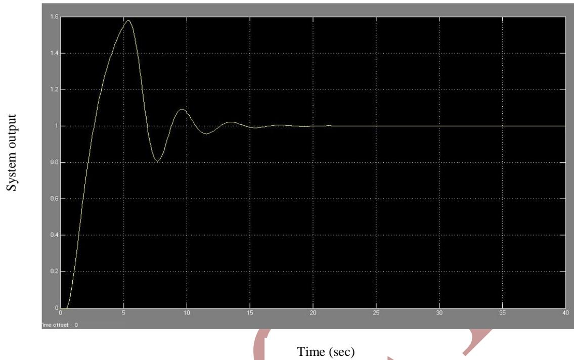
Figure : 2 Step response of process  $P_1(s)$  without anti-windup
