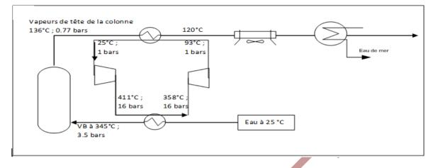
Figure 3 : Location and heat pump operating parameters
