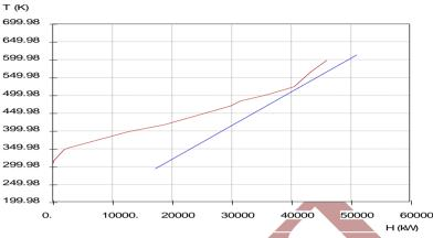
Figure 1: hot and cold composite curves
