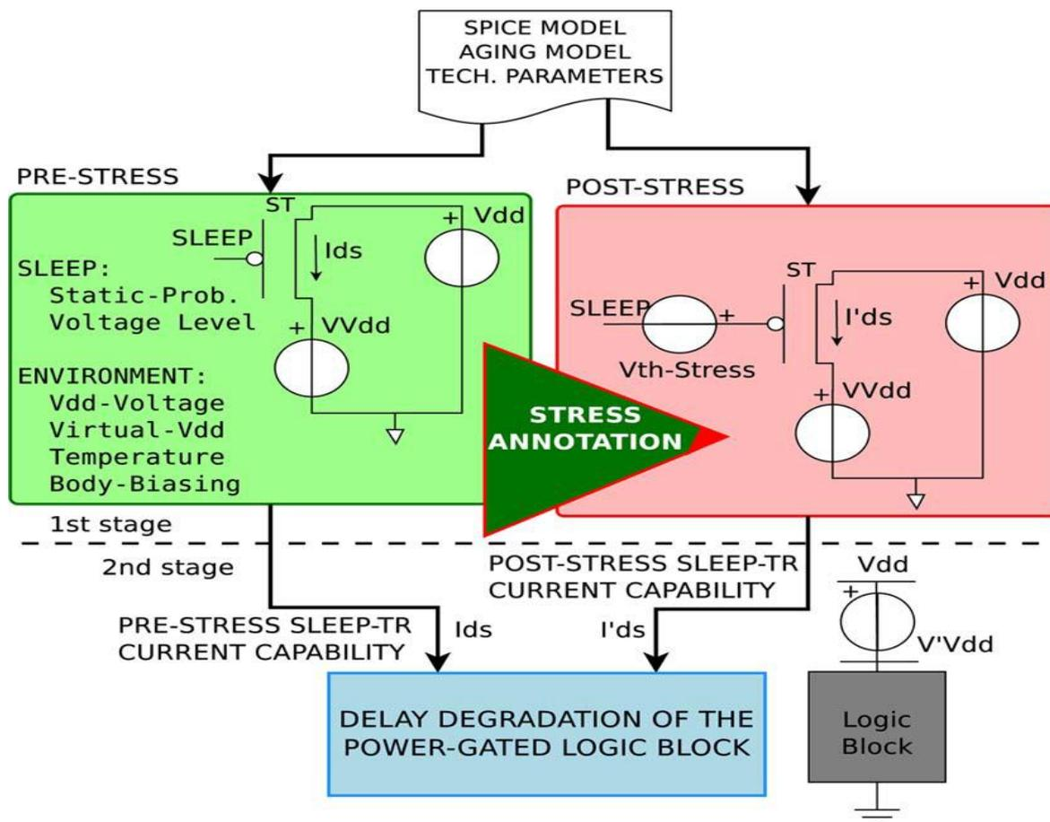
Fig. 1. NBTI-characterization flow for pMOS sleep transistor
