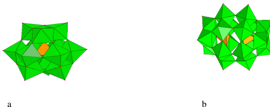
Figure1. - showing the position of heteroatom (a) in Keggin structure (one P-atom) and (b) two P-atoms (yellow colour) in Dawson structure.
