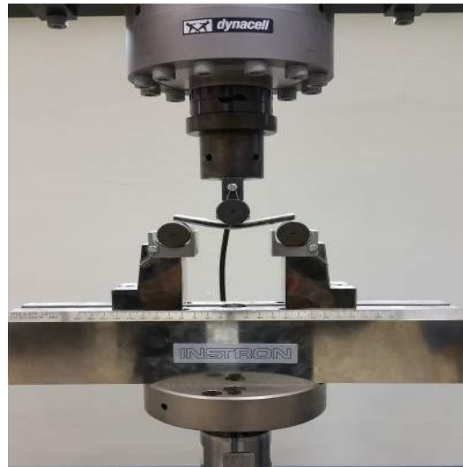
Fig.5 Failure of the component at maximum load
